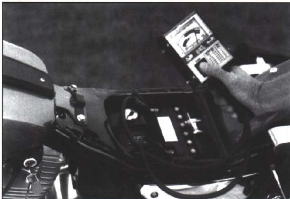
Charging and starting problems can be detected early with a battery tester. Photo courtesy: Associated Equipment Corporation, St. Louis, MO.
