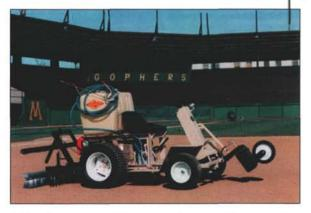
AFM stripes, sprays, and grooms, saving on maintenance time and materials. AFM can stripe several football fields without the need to refill; level and groom athletic fields with a heavy-duty harrow and broom or dragmat; and spray chemicals for weed and insect control. It can also pull a utility trailer or other accessories.
