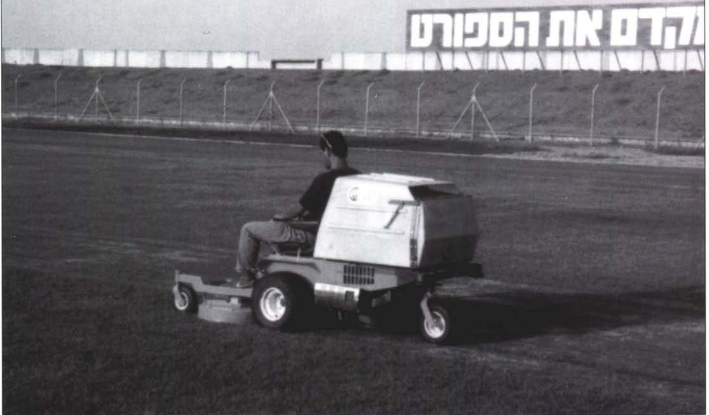
Walker mid-size rotary mower at work on a soccer field in Israel.
