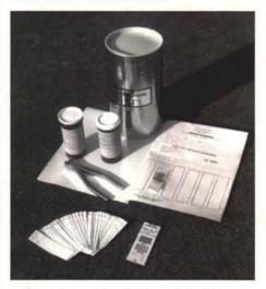
The Tissue Test Kit from Turf-Tec can be used for on-site determinations of the nitrate-nitrogen levels in turfgrass leaves and stems. A color chart shows low, medium, and high in approximate parts per million, which is used to compare with the test. An analysis of the nitratenitrogen can be made in one to five minutes. Full color will appear in approximately 30 minutes.
