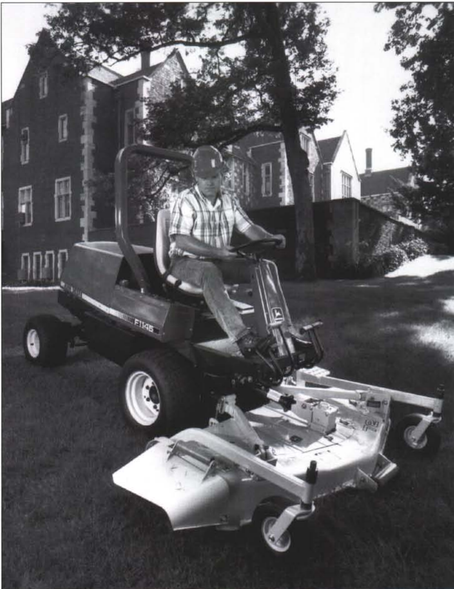
On-demand four-wheel-drive, front differential lock, and roll over protection offer traction and safety on Deere's F1145.
