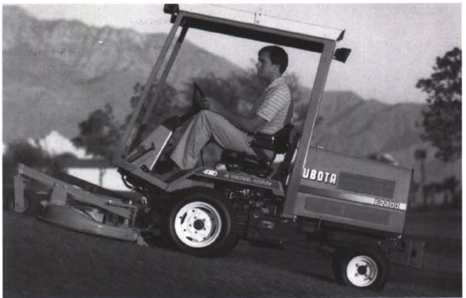
Kubota F2100 sports a low center of gravity and four-wheel-drive for mowing slopes.
