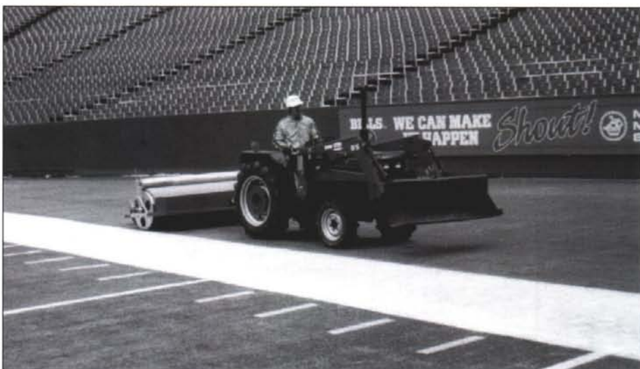
Pull-behind water removal device by Kuranda comes in handy at Buffalo's Rich Stadium.
