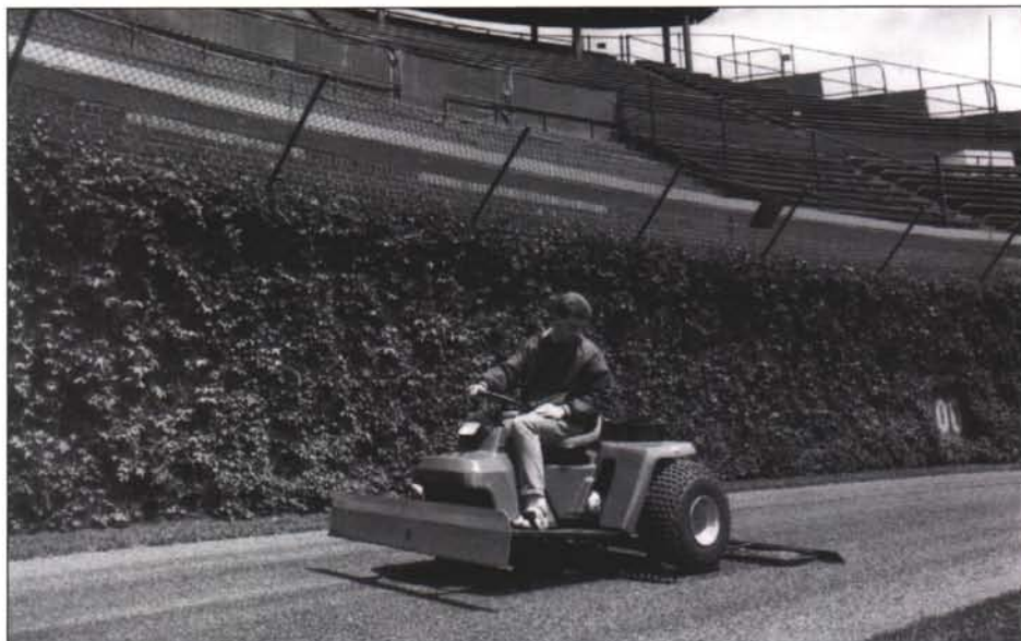
John Deere 1200 Bunker and Field Rake at work on the warning track of Wrigley Field.
