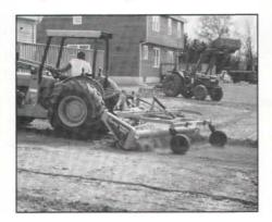
Industrial strength components and simplicity of design permit maximum performance and minimum maintenance. The heart of the system consists of two power-rotated steel rollers mounted above each other and at an angle to the ground. The clockwise rotating bottom roller is built from six-inch,hollow, quarter-wall steel pipe with 3/4-inch steel bars securely welded to it. Rotation is into the grain of rough, packed ground.
