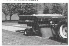
The Mete-R-Matic LA2 Large Area Top Dresser is a front-discharge top dresser. It works with all types of top dressing materials, wet or dry, and can be used with any standard 35 horsepower tractor.
