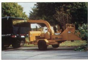
A self-feeding brush chipper, capable of handling material up to 12" in diameter, is now available from Vermeer Mfg. Co. The model 1220 is equipped with a hydrostatically controlled vertical feed roller system. Variable speed control of the rollers ranges from 0-120 fpm. An optional sensor controls the feed to the 37" cutting disc, which has 2 or 4 steel-hardened knives. The 4,480 lb. unit is available with Ford gas engine or Perkins Diesel.
