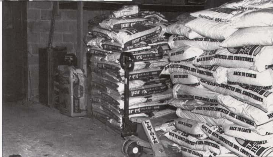
A well-designed fertilizer storage area. Fertilizer is kept off the floor and forklift access is easy.
