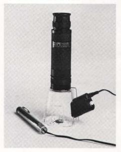
A new portable camera-adaptable macroscope instrument, the Macroscope 25 "H" Kit, has been introduced by RF Inter-Science Co. It combines the Macroscope 25 with the new battery-powered Hi-Intensity Illuminator and a padded carying case. This makes the system a self-contained, field-usable microscope providing wide field magnification of 25X. By adding the optional Macromate I camera adaptor, field photography at 25X is possible without any elaborate set-up.
