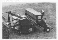
The Olathe Model 71/831 Aerator/Polymer Planter plants water-absorbing polymers that form a subsurface water reservoir where plant roots can absorb water as needed. The Model 71 Aerator cuts grooves in the ground with rotating blades, then the Model 831 Polymer Planter deposits the polymers into the grooves through stationary planter blades. A 48-x-36-inch
