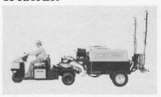
Cushman's 240-gallon sprayer is designed for the fifth wheel attachment to its Turf-Truckster vehicle. It attaches to the vehicle with a two-inch ball hitch.
