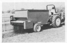
The Bear spreader/topdresser has a five-cubic-yard capacity. Its 60-inch nylon brush spreads various materials evenly and without clumps.
