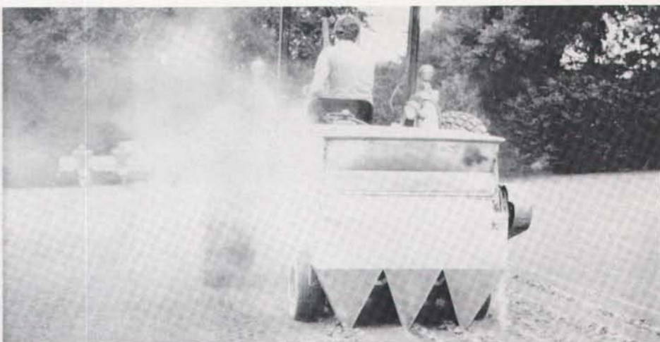
Hopper feeds sand into slits cut by VertiGroove machine.
