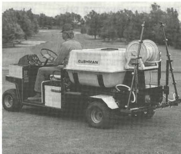
Low profile sprayer on Cushman Turf-Truckster.
