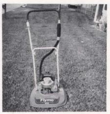
The Flymo GCT 20-inch hovering grasstrimmer has a unique nylon-line cutting system. The line is constructed of long-lasting, triangular monofilament.
