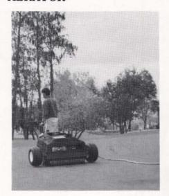
The HydroJect 3000 uses high-velocity water to aerate compacted soils without disturbing their surfaces. The water jet penetrates the surface with a clean entrance hole, approximately the size of that created by an earthworm, and begins to fragment the soil laterally as it penetrates deeper, lifting and shattering the soil underneath. This loosens the soil and leaves channels that are conducive to root growth and water infiltration.
