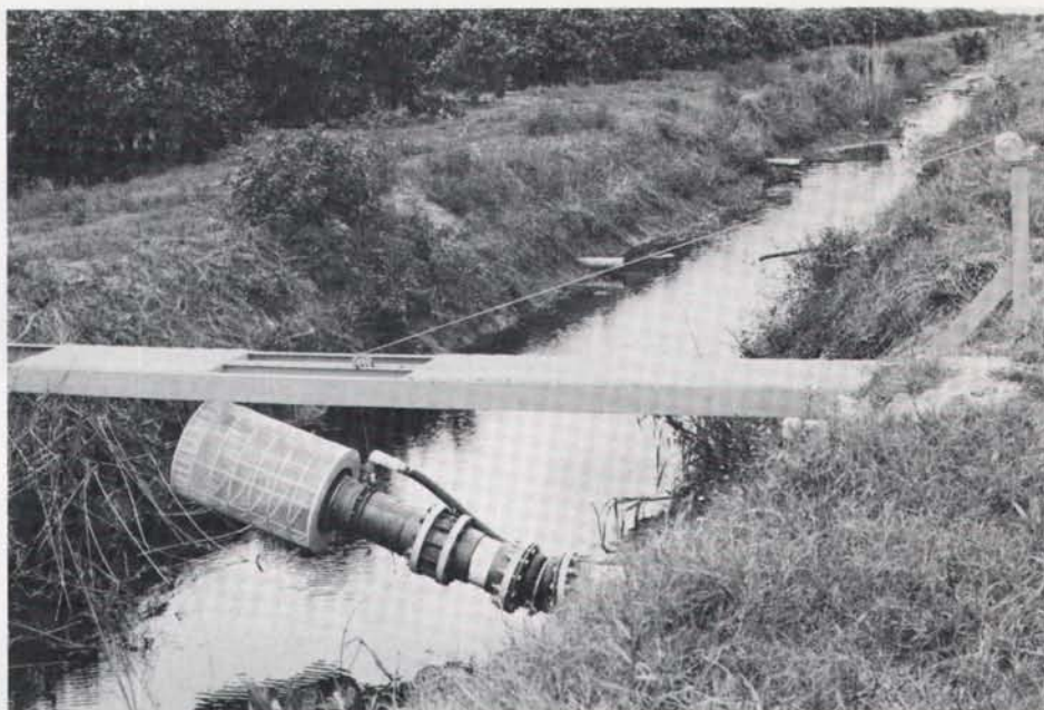
Plum Creek filter uses jets of water to backwash intake screen.
