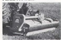
The RHD88 flail mower has an 88-inch cutting width, and is equipped with a 90-hp intermittent (and 60-hp continuous) gearbox, category-four driveline, and a 4-1/2inch cutter shaft. Features include a unitized drive transmission, forged steel gears and shafts, sealed gearbox, shielded drive shaft with slip clutch, and a rigid three-point-hitch frame harness.
