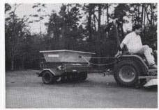
The Olathe Model 23 Topdresser is a tow-behind unit that can be pulled by most utility vehicles and tractors. The maneuverable unit has a 60-inch swath, and evenly distributes topdressing using a high-speed brush to propel it to the base of the turf. Its ground-powered hydraulic drive reduces maintenance problems associated with
