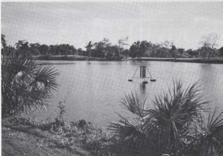
The Pond 1 by Lake Aid Systems is a wind-powered vertical aerator.
