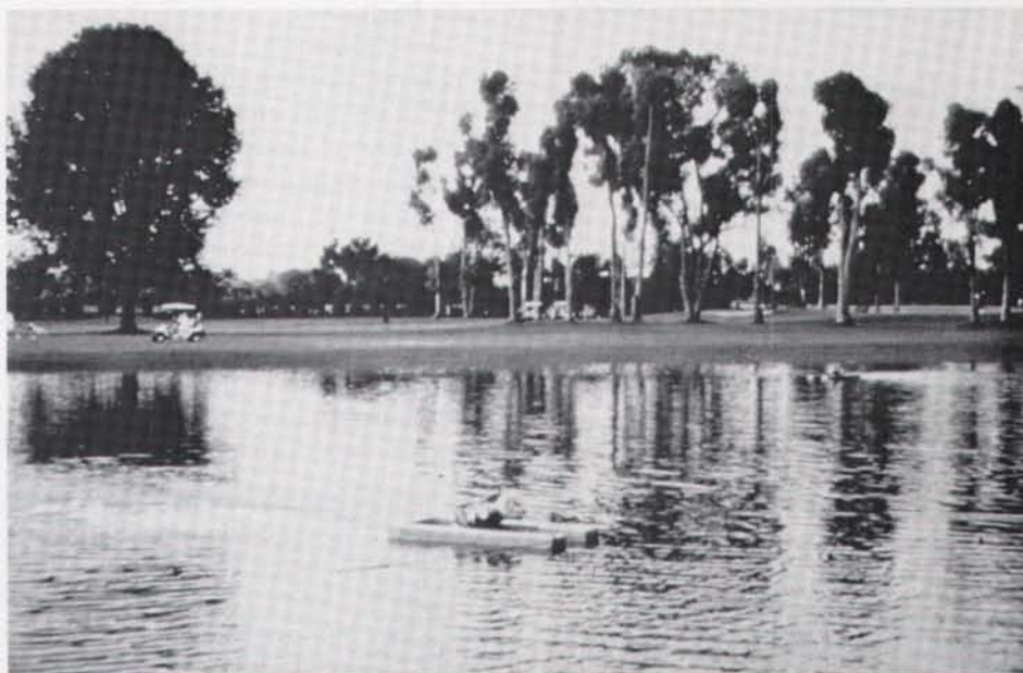
The Toro Aire O 2 is an electrically-powered horizontal aerator.
