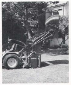
The Seko Model BM27 turf groomer is a power sweeper, mulcher, dethatcher, mower, and roller in one machine. Its 50cubic-foot hopper is available in a ground or high lift dump.
