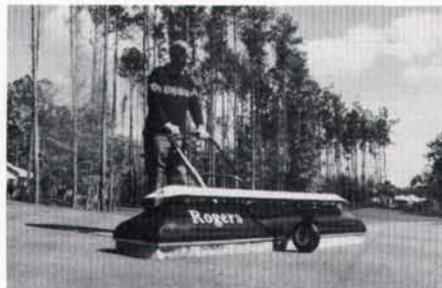
The 80-inch Greensfoil Hosefed Walking Boom has mechanical drift control, which allows spraying in windy conditions. Its advanced airfoil protects the operator and environment and ensures positive drift control.
