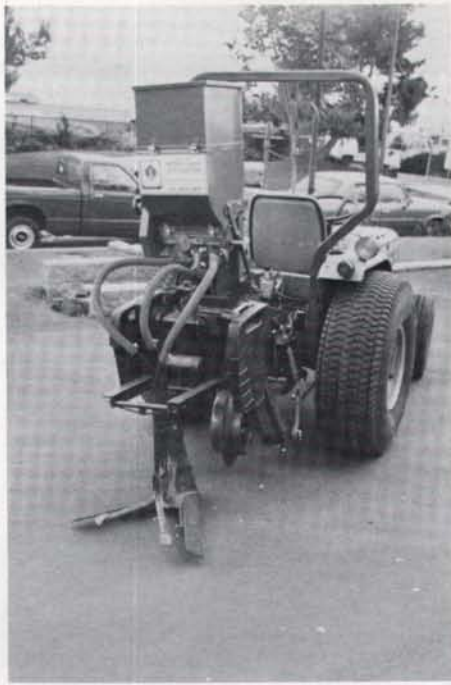
Hydro-Hold Applicator lifts soil and sprays a 28-inch-wide band of dry, synthetic polymer.
