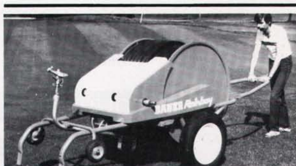
RAINBOY: A Portable Above Ground Automated Sprinkler System.
