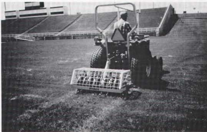
HydroJect 3000 Aerator by Toro uses jets of water to cultivate rootzones.
