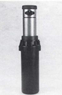
Designed for sports fields, golf courses, cemeteries, and other large turf areas, the I-40-ADS adjustable arc sprinkler can be set at any arc between 40 and 360 degrees. Arc adjusment can easily be made with the water on or off.
