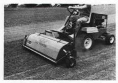
The Model 56 Plug Pulverizer attachment of the Toro Groundsmaster 300 series helps pulverize and top dress after aeration using the close center coring aerators. Only rubber fingers come in contact with the ground, as opposed to steel hammer blades. Plugs are lifted off the turf and bat-
