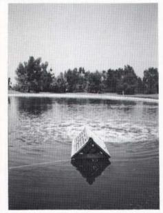
The Aire-O2 Golfwater aeration system is designed to control water quality problems and restore water quality in golf course ponds. By thoroughly aerating and circulating pond water, the system controls algae, scum, stagnation, and their accompanying odors.
