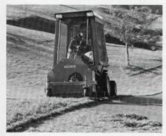
The F2400 front mower is equipped with a 24-hp, four-cycle, three-cylinder, vertical liquid-cooled diesel engine. The unit's hydrostatic transmission works together with its front differential lock and four-wheel-drive to provide traction and smooth operation on uneven or slick terrain. In addition, the hydrostatic transmission per-
