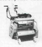
The Olathe Model 84 Walk-Behind Aerator/Slit Seeder's reverse-action clutch increases operator maneuverability and ease of operation. The unit is powered by an 18-hp engine.
