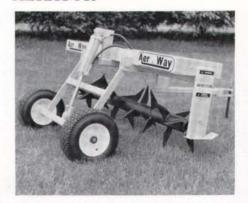
The new Aer-Way pull-type hydraulic lift shatter tine aerator from Holland Equipment Ltd. is designed for low-horsepower tractors and tractors without a three-point hitch attachment. Hydraulic outlets are required to operate this unit. The tongue is easily attached to the drawbar and the frame is hydraulically lowered or raised for transportation or clearance of obstructions. Aeration blades are available in 4-1/2-, 6-1/2-, and eight-inch lengths.
