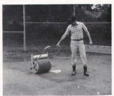
Kuranda's Super Sopper water removal machines quickly remove puddles from soggy clay infields. Using a sponge-covered roller with an internal storage tank, they can pick up 3/4 of an inch of water per pass from grass, artificial turf, and sandy infields. Six different models are available. They can remove from 100 to 4,000 gallons of water per hour from any playing surface.
