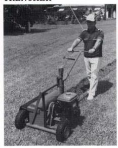
Powered by a 4.6-hp Wisconsin engine. the Model K-T 200 double V-belt drive portable trencher can dig 20 to 30 feet of two-inch-wide trench per minute. Digging depth is adjustable to eight inches.
