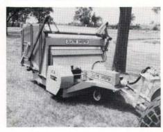
Models 166E and 166HL Olathe Turf Sweepers are designed to follow ground contours and avoid obstructions while picking up grass clippings, leaves, twigs, bottles, cans, and other debris. The units are PTO-powered and equipped with the Sure Grip rubber finger pickup system which can handle wet or dry material.
