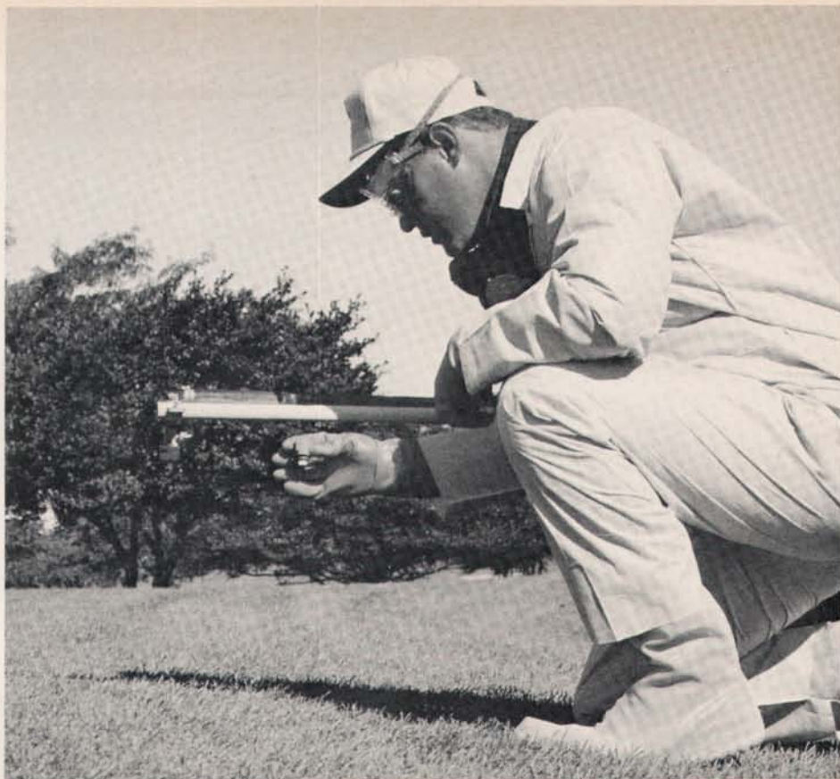
Nozzles should be inspected often and replaced if necessary.
