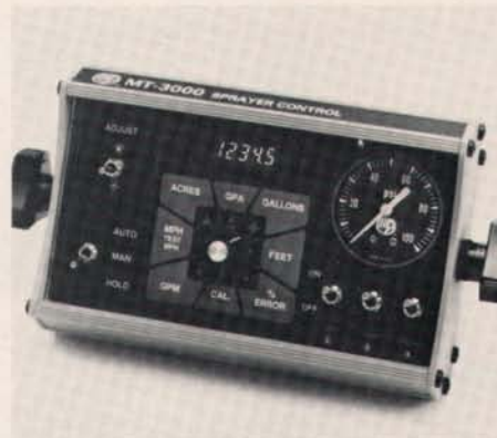
Sprayer control system by Micro-Trak monitors flow rate and ground speed to maintain a desired application rate.
