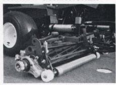
Jacobsen offers the Turf Groomer fairway conditioner, which has a large front roller and thick cutting blades for greater strength and durability. Two blade spacings are available. Its drive system has a tough, one-inch drive belt that is protected from debris by a sealed housing. The cover is easily removed for inspections and adjustments.
