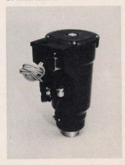
A "family" of valve-in-head sprinklers has been introduced by Buckner. Blending some of the best new technologies with the reliability of the old, the sprinklers combine a cam drive sprinkler and piston valve into a compact package of high-tech plastics, bronze, and stainless steel.
