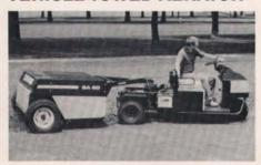
Up to 1.3 acres per hour can be aerated by the GA 60 Fairway Aerator. The vehicle-towed unit has a 60-inch swath with a 2½-x4½-inch coring pattern, at an aerating depth to four inches.
