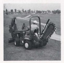
Trenches six to 12 inches wide can be dug to a depth of 63 inches with the Ditch Witch Model 3500 all-hydraulic trencher. The Model 3500 also has a 64-inch-wide, four-way (six-way optional) backfill blade, designed to roll, rather than push, spoil into a trench for easy, efficient backfilling.
