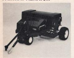
Capable of aerating up to 50,000 square feet an hour, the Toro Fairway Aerator has a five-foot coring swath. Coring depth is controlled with adjustment brackets on either side of the unit. The coring unit can be easily adjusted down to five inches in depth, with the two-tine head, and down to three inches with the six-tine head.
