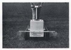
The spreader is used to apply liquid fertilizers, herbicides, fungicides, insecticides, and growth regulators. Its twin wheel pumps spray a six-foot-wide fan of solution, with an overlap at the center, at a rate of 1,000 square feet per gallon.
