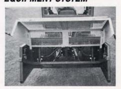
With its two quick-release couplers and hydraulically powered by a tractor, the Modus T Mainframe System can accommodate a variety of tractor-pulled turf care equipment. Tool options include a mole plough, topdresser, athletic field conditioner, a sweeper (verti-cut or flail head are also optional), an athletic field conditioner, and a scarcifier.
