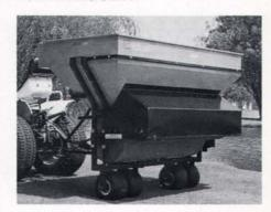
Constructed of tubular steel and zinc annealed sheet metal, the Spread Master topdresser is a tractor-pulled, all-hydraulic drive machine designed for durability.
