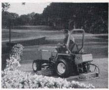
Featuring a self-contained hydraulic system powered by 540-rpm PTO drive, the 303 and 305 hydraulic reel mowers from John Deere provide an efficient, high-quality cut. Each has a large hydraulic tank with a full-flow filtration system to help keep its oil clean and cool.
