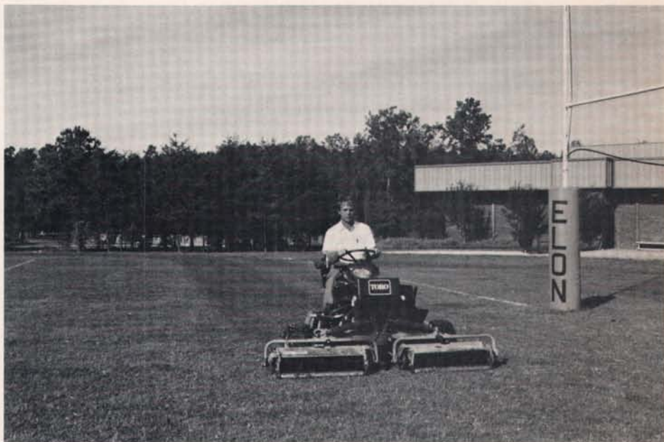
The Tifway bermudagrass athletic fields are cut three times each week with a triplex reel mower.
