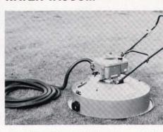
The Hover Dry is a lightweight, portable, self-contained machine that removes surface water at a rate of up to 80 gallons per
