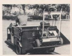
The unit attaches to the stake pockets of the Cushman Turf-Truckster short box, where it is secured by pins. To load the carrier, the operator merely raises the Turf-Truckster box, which lowers the equipment carrier to ground level. A mower or other equipment can then be rolled onto the carrier. Lowering the dump box raises the carrier and tilts it slightly forward to hold the equipment during transit.
