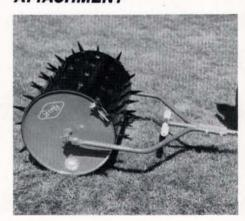
A clamp-on aerator attachment will convert a Gandy Company 18-by-24-inch lawn roller into a durable core aerator.
