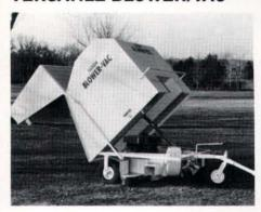
The Saxon Blower/Vac II, from D.E. Wolfe Metal Fab Company, vacuums into four-foot-wide spaces, enabling it to fit easily between shrubs and trees, through gates, and in various tight spots. The powerful unit picks up leaves, clippings, thatch debris, pine needles, and parking-lot trash.
