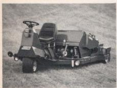
Powered by a 20-hp Kohler engine, the Riding Aerator from Salsco, Inc., is designed for greens, tees, fairways, sports fields, and other large turf areas. With variable core spacing from one to six inches, the unit is capable of aerating over 60,000 square feet per hour.
