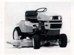
Ariens has introduced a pair of versatile turf tractors, the 20-hp GT20 and the 18-hp HT18. Both are powered by twin-cylinder Kohler electric-start engines.
