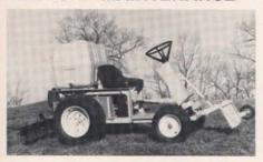
The versatile Kromer utility vehicle can apply paint for line-marking athletic fields, dispense chemicals for weed and insect control, or pull cultivating and leveling attachments for conditioning baseball diamonds.
