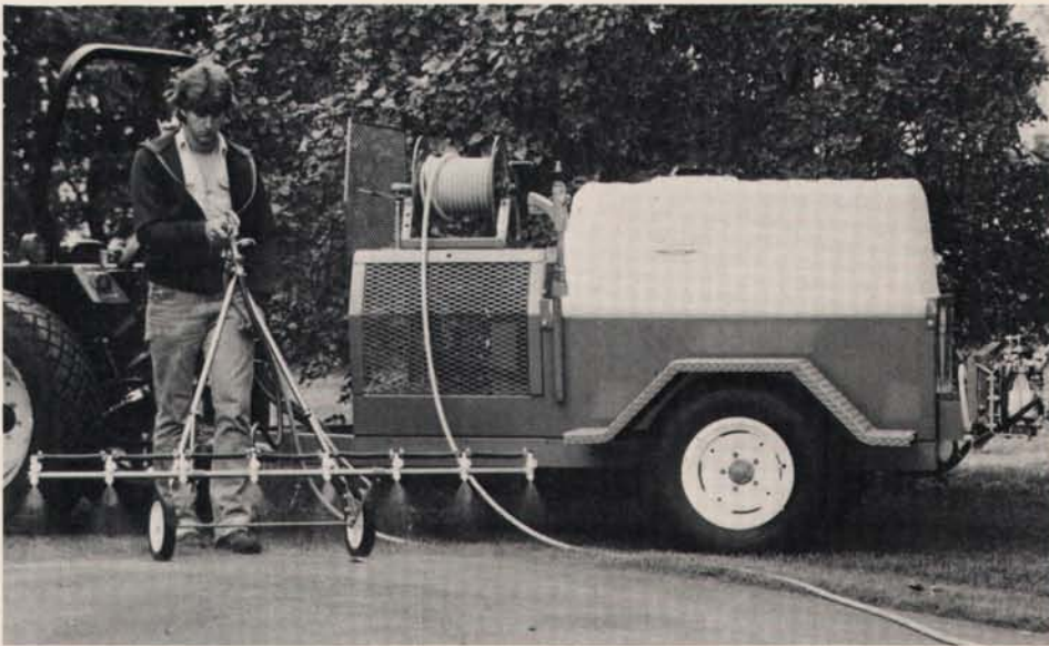
Boom sprayers and spray pattern indicators keep overlap to a minimum.
