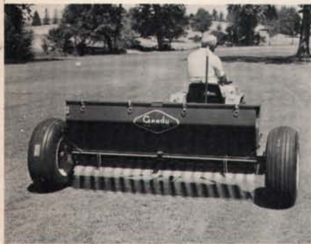
Drop spreaders are preferred over cyclone-type spreaders for granular applications on fine turf.
