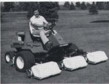
With on-demand four-wheel drive the Jacobsen LF-100 five-gang fairway mower can climb hills without damaging turf from wheel spin and slippage.
