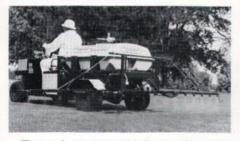
Two turf sprayers with low profile tanks are now available from the Cushman Division of Outboard Marine Corporation. They come in either a 120- or 150-gallon tank size, and both are designed to mount easily on the Cushman Turf-Truckster chassis with the pin-disconnect system.
