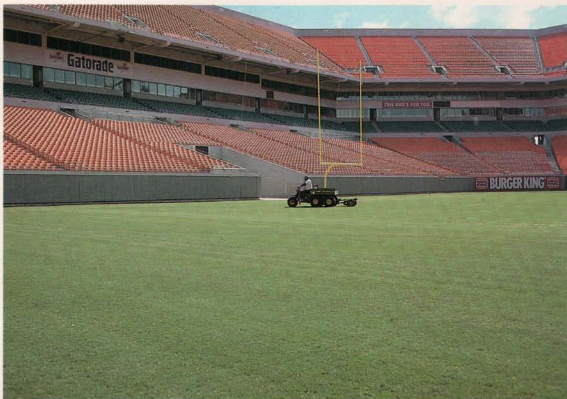
Mascaro's invention, the Vertislicer, was used to break through a subsurface layer and to encourage root growth.
