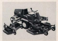
Responding to the turf-maintenance needs of professional groundskeepers, The Toro Company has introduced a productive, maneuverable large-scale mower—the Groundsmaster 580-D high-capacity turf mower.
