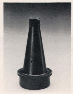
The DRHA-1 DR Hose Adapter enables Rain Bird electric valve-in-head DR rotors to operate as quick-coupling valves on the golf course. The adapter may be quickly installed in the field by replacing the rotor's internal sprinkler assembly.
