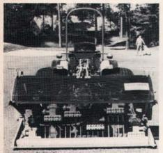
The Model 105.145 Verti-Drain deep-tined aerator can alleviate the most difficult soil-compaction problems.
