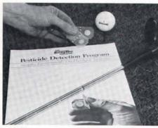
Golf course supertindendents can monitor applicator exposure to insecticides in three minutes with a test kit from EnzyTec, Inc. Originally developed by Midwest Research Institute under contract from the U.S. Army, the test detects 80 percent of the insecticides registered for use in the U.S.: namely the carbamate, thiophosphate, and organophosphate insecticides.
