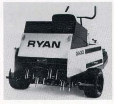
OMC Lincoln now offers a riding aerator that allows the operator to vary the core
