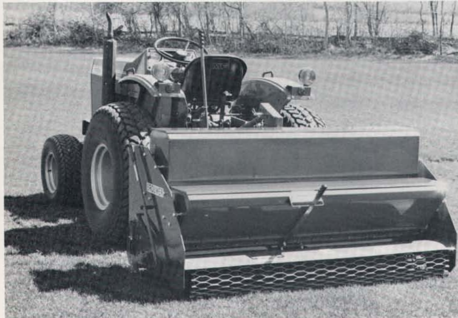
Broower seeder used for large areas with prepared soil.
