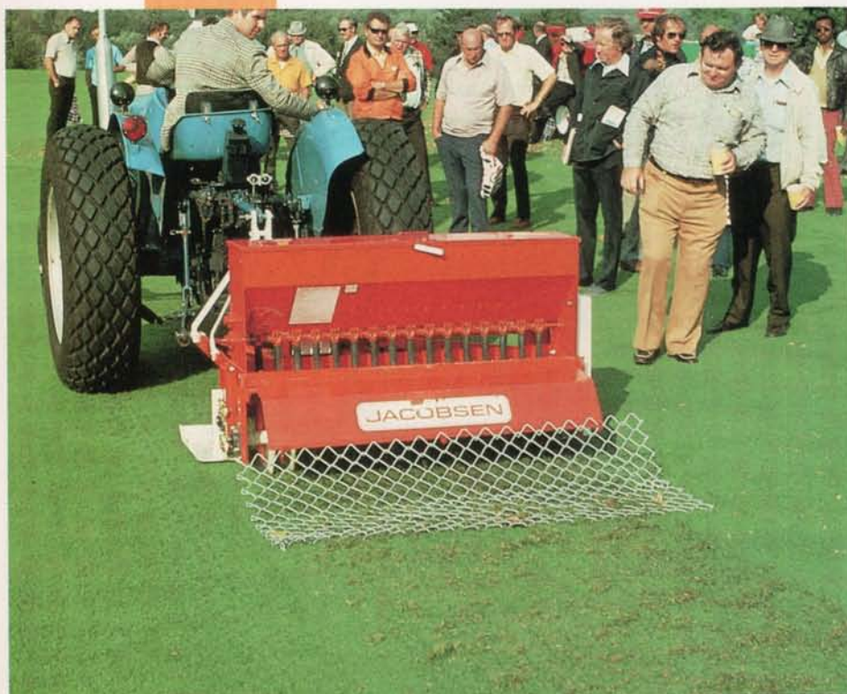
Large area overseeder assures better soil contact and higher germination.
