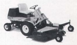
ANSWER: The Cushman 809. This new gasoline water-cooled Front Line® Mower features a 27 hp., 3-cylinder Teledyne-Wisconsin engine that cuts through the toughest, tallest grasses with power to spare. It's quiet and it stays cool for years of top-cutting performance. For all the facts, return the reader service card in this publication today.
