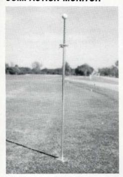
Soil hardness can be easily measured in the field or on the golf course with the Turf-Tec Penetrometer. The device is a precision instrument that uses gravity to provide soil hardness readings from zero to 100 percent compaction.
