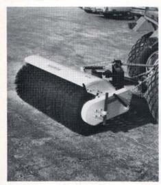
Turf tractors with 540 PTO and a threepoint hitch can be put to work sweeping turf or pavement with the Sweepster RHFA. The unit windrows debris or snow outside the left or right rear tire with the tractor moving forward. A full 30 degree sweeping angle is provided with minimum vibration and maximum component life.
