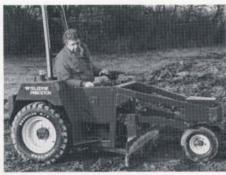
wheel design allow the operator to grade within a one-half inch of any structure, wall, pipe or tree and turn within the length of the unit. Variable speed and reliable torque hubs provide the extra traction needed for grading work.
