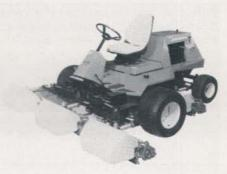
Jacobsen has added two more gangs to light-weight fairway mowing with its LF-100 five-gang reel mower. The unit offers precision mowing and low ground pressure previously available only on triplex greens mowers. It cuts a 100 inch swath at speeds up to five mph for higher productivity than triplex mowers.
