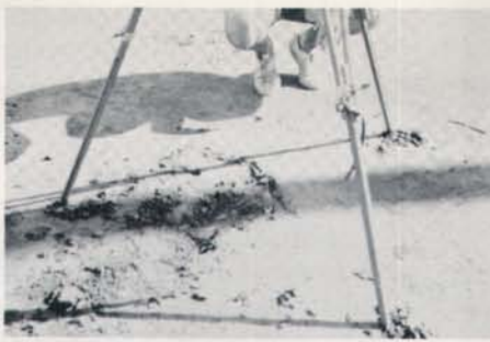
The transit's plumb bob must fall directly over the apex of home plate.
