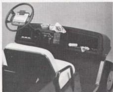
The 1988 four-wheel PARCARS feature a new automotive-style console/ dashboard. A convenient dash-mounted key switch controls forward and reverse directions. You choose the direction the golf car goes with the turn of the key.
