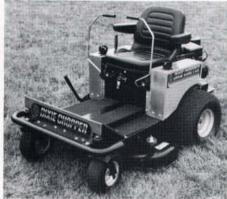
Dixie Chopper mowers now feature full hydrostatic drives. Available in 42-inch, 50inch, and 60-inch sizes, these new models eliminate all drive chains and sprockets.
