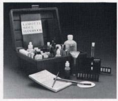
The Turf Lab Model TL-1 test kit provides on-site evaluations of turf- grass soils. An improved colorimetric test method is used to achieve quantitative measurements for pH and phosphorous. Utilizing an Octa-Slide comparator, permanent translucent color standards are compared to clear liquid test samples for more accurate readings.
