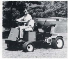
The versatility of Hahn's Multi-Pro 44 turf vehicle has been expanded with the addition of a spreader/topdresser attachment. The unit can distribute 600 pounds of dry sand per minute in a 12- to 20-foot-wide swath or fertilizer in a 45-foot-wide pattern.
