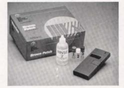
turf and antibodies produced by plants to fight them. The company has reduced a laboratory procedure down to a simple litmus test in which a test strip is inserted into a solution of ground-up turfgrass tissue. A small meter is used to read the darkness of the strip to reveal the level of fungi present.
