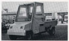
The GX-20 is a ruggedly constructed small pickup for campus, golf course or park light hauling jobs from Chikusui. Less than 48 inches wide and ten feet long, the vehicle can carry a payload of nearly 1,800 pounds. Loads are easily dumped with the hydraulic tipping bed.
