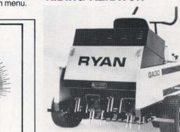
Clean, vertical-coring action and variable core spacing are two major features of the new Ryan GA-30 riding aerator. The operator can change the core spacing anywhere between  $2\frac{1}{2} \times 1$  inches to  $2\frac{1}{2} \times 5$ inches with a hand lever while aerating. Depending upon the tines and soil condition, the aerator can penetrate up to  $3\frac{3}{4}$  inches deep. At the five inch spacing the GA-30 can create 11 holes per square foot over a 28,000 square foot area in an hour.
