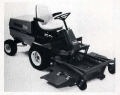
A power-assisted four-link steering system and other design improvements resulting from 20 years of development work by Toro make its new 220-D intermediate size trim mower highly maneuverable and productive. The company has increased handling ease while lowering maintenance difficulty with its compact, liquid-cooled trim mower.
