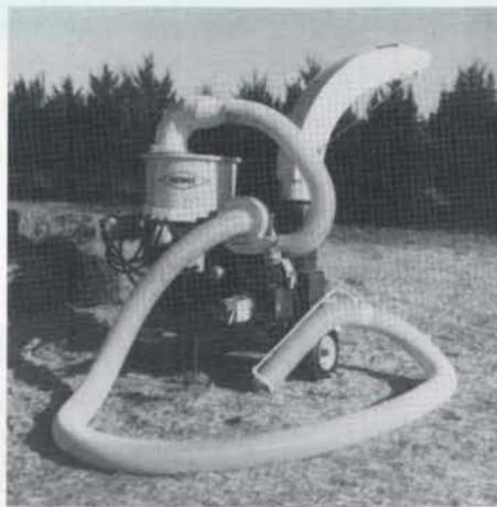
Henke Machine has increased the versatility of its chipper/grinder by adding a blower assembly with a six-inch-diameter, 30-foot-long hose. Not only does the unit grind up limbs and lumber, the blower and hose assembly can be used to distribute mulch or to vacuum leaves and debris for grinding.
