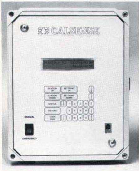
The Calsense 1000 irrigation control computer working in conjunction with field moisture sensors can reduce water usage by 30 percent or more according to California Sensor Corp.
