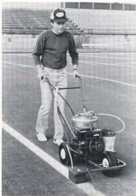
Pioneer Manufacturing Co. of Cleveland, OH has introduced the Brite Striper Model 1500 gasoline-powered line striper.
