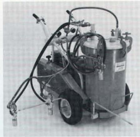
EZ-Liner Industries has developed a new self-propelled option for both its single and dual version of Model 588 EZ-Liner. The unit is belt driven with fully pneumatic controls. Its double handle and fixed rear caster allow for maximum maneuverability and straight line operation. The dual gun set-up with adjustable stripe width from two- to six-inches, makes double-line marking quick and easy.
