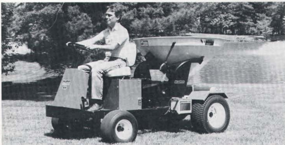
Large hopper pendulum spreader from Hahn is a fast way to topdress lightly.
