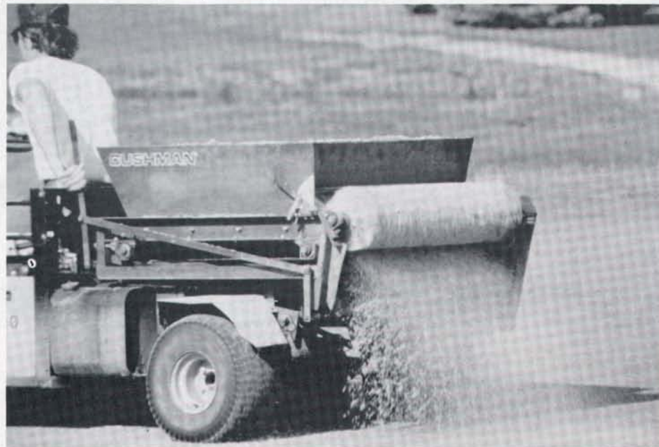
Brush on Cushman topdresser distributes mix evenly and breaks up clumps.
