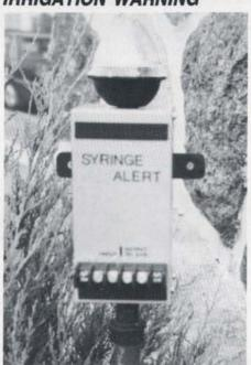
An electronic warning device, Syringe-Alert, is designed to forewarn golfers of the opening of any electrically controlled irrigation valve.
