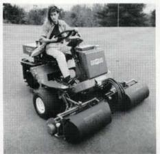
New from Bunton, this triplex greensmower is available with a cool-running, 18hp, twin-cylinder, aluminum-block Onan engine with cast-iron sleeves, or with an optional 16.5-hp, three-cylinder, water-cooled Kubota diesel engine.
