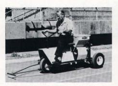
marker holds up to 125 pounds of chalk or ten gallons of water-based paint to mark large fields or tracks quickly without stopping to refill.
