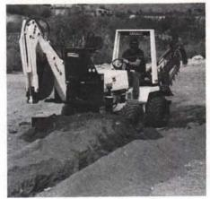
Matching trenching speed to soil conditions is simple with the Bobcat T-135. Both the ground speed and trenching speed are infinitely variable in both forward and reverse due to hydrostatic drive, a unique feature for trenchers in the 35 hp class.
