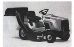
Yamaha has introduced the first model in a new line of turf tractors. The YT3600 features a counter-balanced 12 hp OHV engine, an automotive-type drive shaft delivering power to a hydrostatic transmission, single-lever control, pinion-and-sector steering and electric power take-off to drive attachments.
