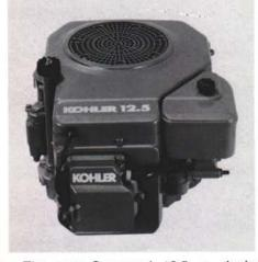
The new Command 12.5, a single cylinder, vertical shaft engine from Kohler provides the power and performance and smoothness of twin-cylinder engines in its class. A computer designed balance shaft reduces vibration while hydraulic valve lifters control operational noise and reduce maintenance.
