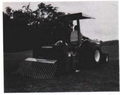
Increase seed germination rates when seeding bare ground or overseeding existing turf with Jacobsen's 548-100 Seeder. Sixteen floating discs follow the contour of the ground and slice grooves in a 48-inch-wide swath. The seed is automatically dropped from a large hopper into the grooves for proper seed/soil contact. A Flo-Rate gauge accurately controles seeding rate.
