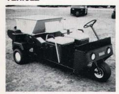
E-Z-Go has built the GXT-1500 turf vehicle to withstand years of daily use at universities, parks and golf courses. Rugged, diamond-plated steel panels secured to a tubular-steel frame enable the vehicle to carry up to 1,500 pounds of cargo. An 18-hp, two-cylinder engine drives the automotive-type, fully-synchronized five-speed transmission. A single shift lever makes the vehicle easy to drive.
