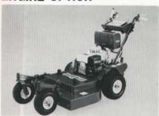
The Honda GXV340 overhead-valve, fourstroke engine is now available as an engine option on Bunton's 36-inch to 52-inch commercial mowers. The II hp overheadvalve, vertical-shaft engine uses up to 30 percent less gas and oil and weighs as much as 25 percent less than comparable sidevalve engines.
