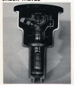
Buckner's 10600 Series Rotary Pop-up Sprinkler with Check Valve saves water and minimizes soil erosion in a wide variety of irrigation applications. The innovative, integral check valve feature reduces low head drainage caused by elevation differences.
