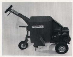
Rotating, drill-like tines on the Promax aerator make vertical holes up to four inches deep in the hardest soils. Designed for small, compacted turf areas, the 22-inch-wide aerator produces shavings which decompose rapidly instead of soil cores.
