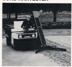
Aeration cores can now be picked up mechanically from golf course greens with the Cushman Core Harvester. Two steel blades gather cores in a 55-inch-wide swath and funnel them onto a rubber conveyor belt for removal. The hydraulically-powered unit is designed to be mounted on three- or four-wheel Cushman Turf-Trucksters equipped
