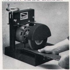
Sharp blades allow rotary mowers to cut turf cleanly without ripping the foliage. The Rotary Blade Grinder accurately sharpens both right or left hand blades to the correct bevel with a fine hollow grind for maximum cutting effectiveness.
